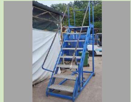
Racking Stair 291cm (H) x 180cm (L) x 70cm (W) Quantity: 1 unit Approx. weight: 64.5kg
